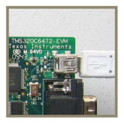
Connect the USB miniB cable to J7 plug for on board embedded emulation, as shown in figure. (For use with CCS debugger only)
